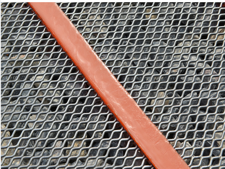
Square self-cleaning screen with polyurethane bands
